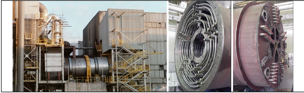
Figure 2: Kumera steam dryer in Pirdop
