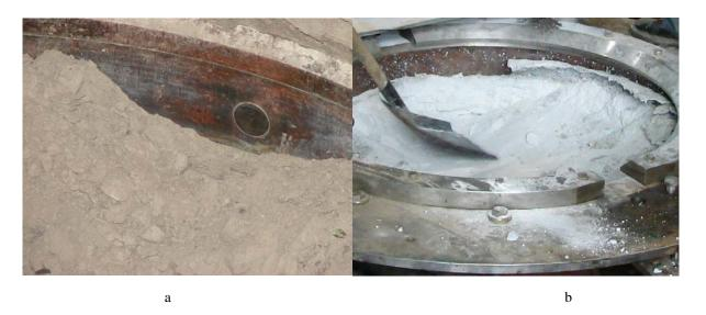
Fig.1 The view of slag bath in the mold of the 920 mm diameter after cooling (a) without metal remelting and after ingot melting (b).
