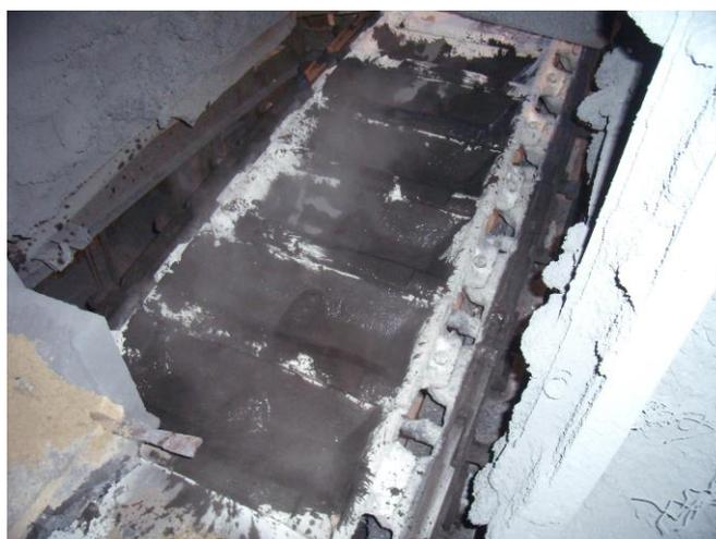
**Figure 2.** Treatment of molds of casting machine by antistick coating based on silica fume (dust of dry gas cleaning).
