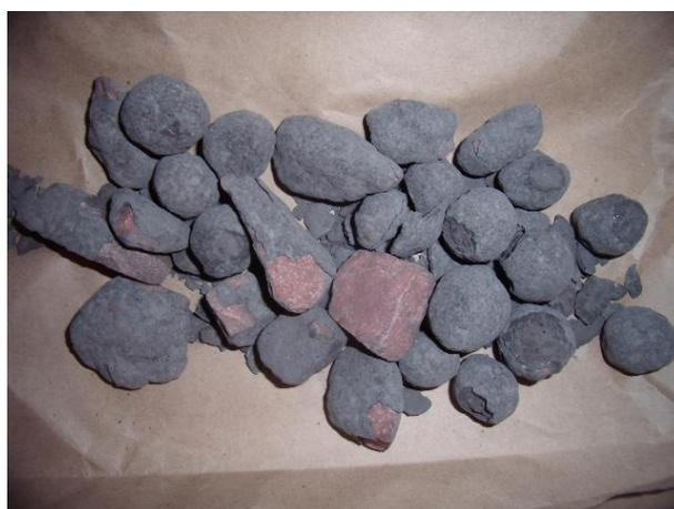
**Figure 4:** The pellets with the core of quartzite pelletizing, after drying
