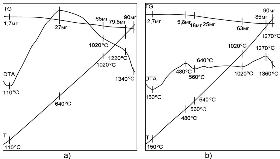
**Figure 1:** Thermogravimetric curves of sintered ore
