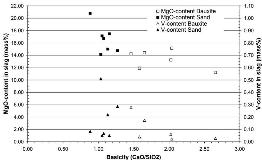
**Figure 3:** MgO-content in the slag as a function of slag basicity ( $\text{CaO/SiO}_2$ ).
