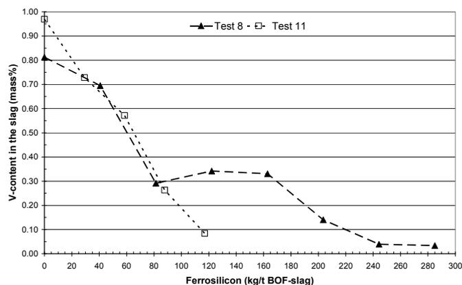
**Figure 5:** Final reduction by injection of FeSi in test 8 (into the metal phase) and in test 11 (into the slag phase).
