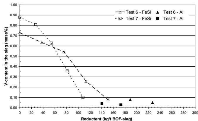
**Figure 7:** Final reduction by injection of both FeSi and Al in the slag in test 6 and 7.
