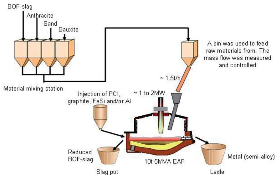
**Figure 1:** Schematically drawing of the experimental setup using a 5 MVA AC furnace with MgO based lining as the basic equipment for BOF-slag reduction.
