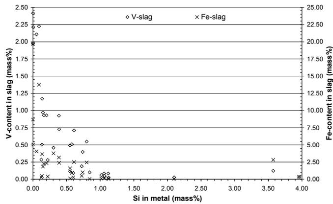
**Figure 4:** The V- and Fe-content in slag as a function of the Si-content in the metal.
