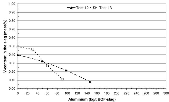
**Figure 6:** Final reduction by injection of Al in the slag in test 12 and 13.
