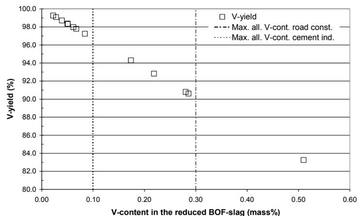
**Figure 2:** The V-yield as a function of the V-content in the final slag.
