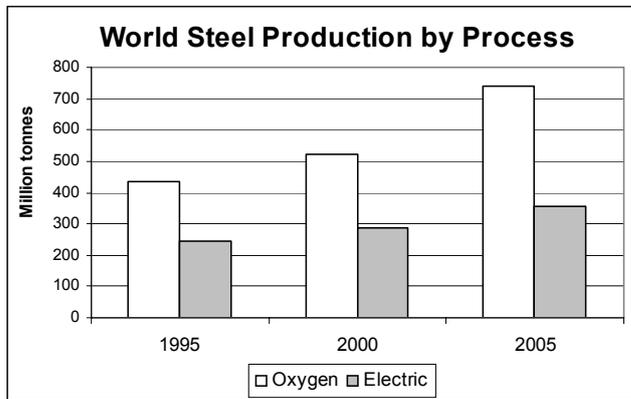
The oxygen route still dominates steel production, despite expectations that the lower cost electric arc route would gain more share. Oxygen steelmaking accounted for 67% of the world total in 2005, compared to 64% in 1995 and 65% in 2000. (Data are from the International Iron & Steel Institute.)
