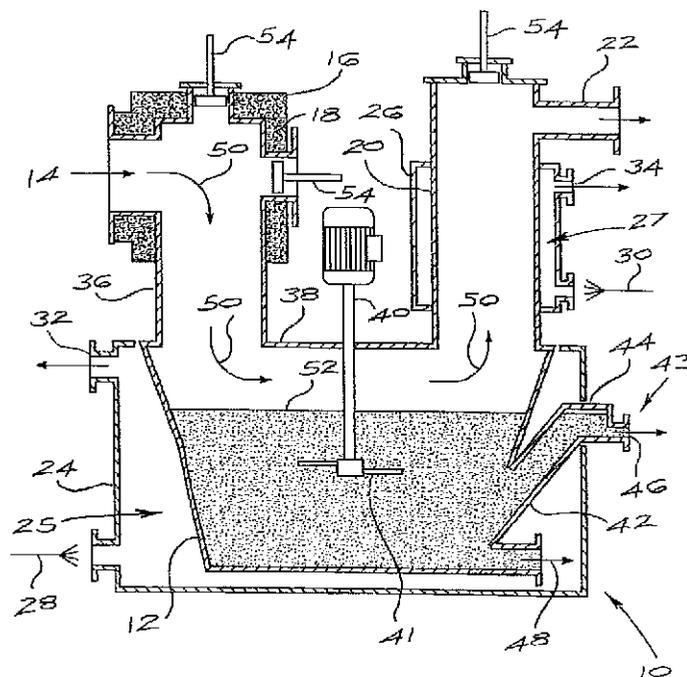
(57) Abstract: Liquid metal is continuously recovered by condensing metal vapour in a sealed system, more or less at atmospheric pressure, and collecting liquid metal in a crucible. The contents of the crucible are agitated and the temperature is controlled to prevent the liquid metal from solidifying. Liquid metal and dross are tapped from the crucible.
