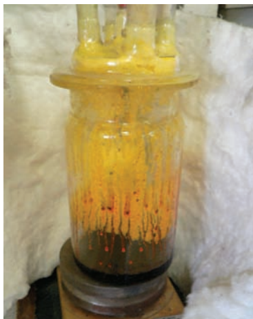
Figure 11—Sulphidation test rig with test sample inserted. Sulphur condensing and running down to liquid bath
