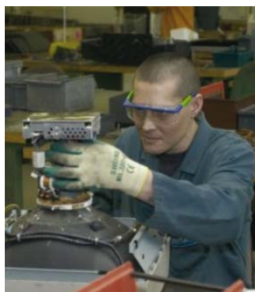
Figure 2: CTR removal in the dismantling step: safe practice in Switzerland (left), hazardous practice in China (right)
