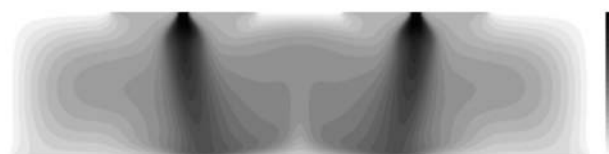
Figure 21—Temperature field, electrode separation 8 cm, M configuration
