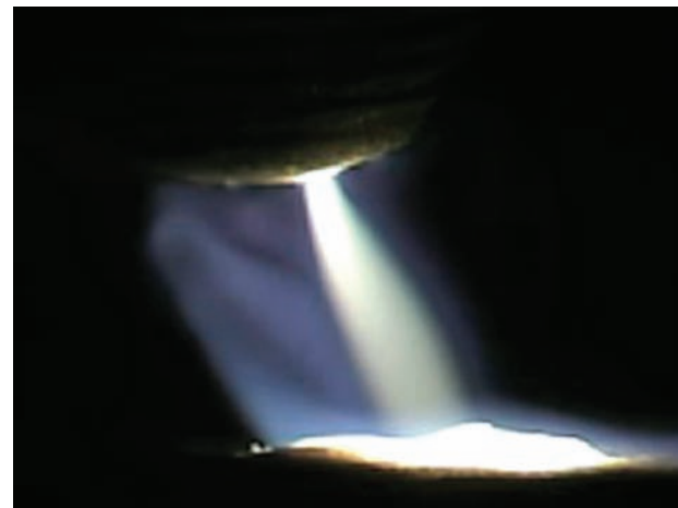
Figure 3—Traditional polarity (cathode electrode) arc, 1 kA, ~80 V, 5 cm length
