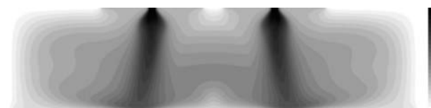
Figure 13—Temperature field, electrode separation 6 cm, dual-electrode
