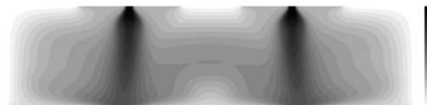
Figure 14—Temperature field, electrode separation 8 cm, dual-electrode
