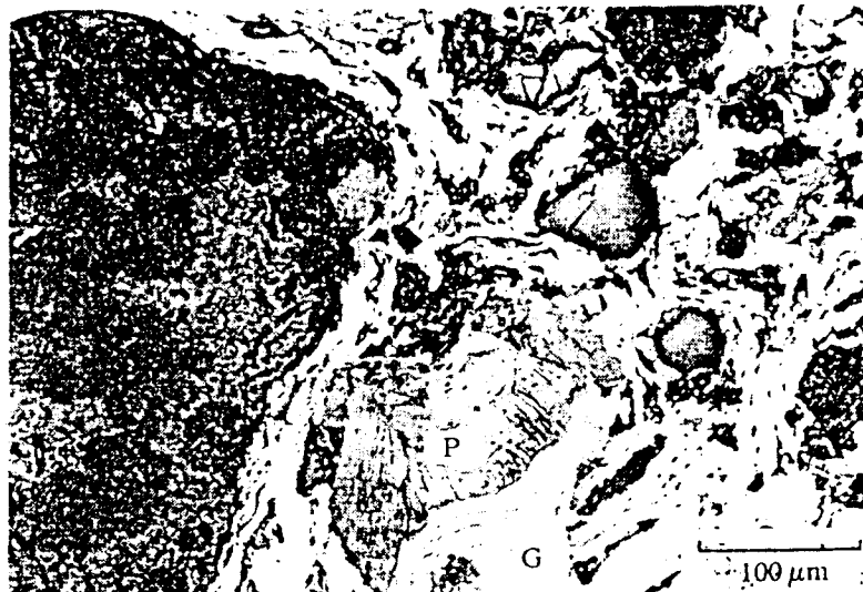
Fig. 16. The optical microstructure of magnesia-graphite conducting hearth refractory. The continuity of the graphite network (G) around the grains of periclase (P) can be seen
