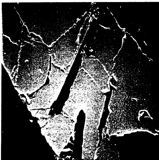
Fig. 13. Metallographic characteristics of metal carbide in the lower region of locality 1/F/1. Flakes or lamellae of graphite that have exsolved from the carbide phase can be seen. (Scanning electron micrograph, polished sample, magnification 40 X)
